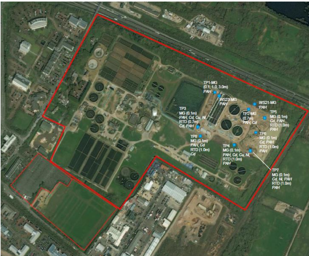
Above: Locations where soil leachate contamination has been identified in previous site investigations
